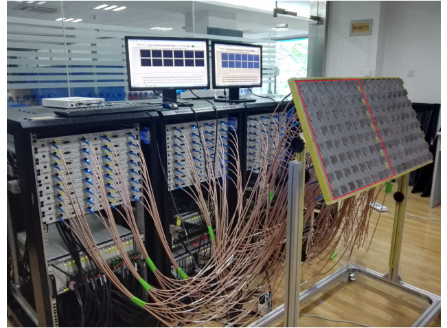
Figure 4. Measurement system and BS antenna array.
